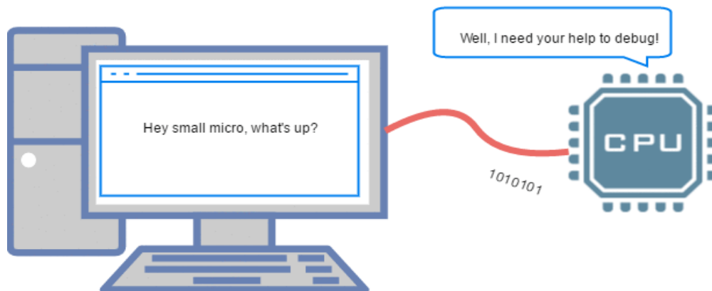
Figure 1: Serial Communication of Microcontroller with PC for Troubleshooting
