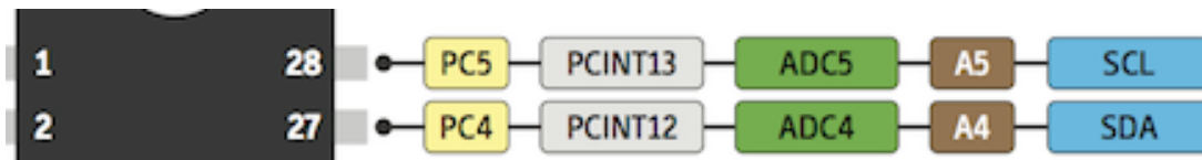
Figure 6: ATmega328P TWI SDA and SCL Pins
