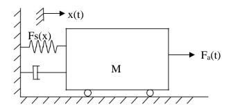
$a=dv(t)/dt = d^2x(t)/dt^2$  is the acceleration
