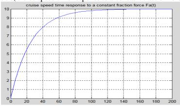
In the above program the behavior of a car speed is shown in which the car starts with rest position, after that it attains its maximum speed so that it reaches its maximum limit then after that its speed becomes constant throughout the time.
