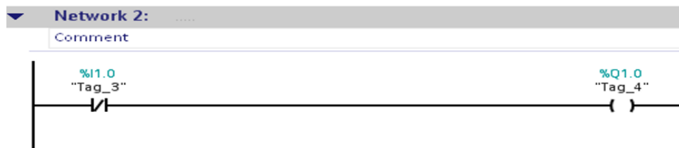
Fig.3 I/O Addresses are in green whereas Tag Names are in black. Remember if you have made mistake in writing I/O address, it turns red.
