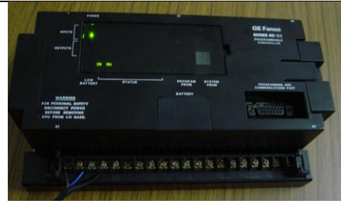
Fig.6: General Electric PLC
