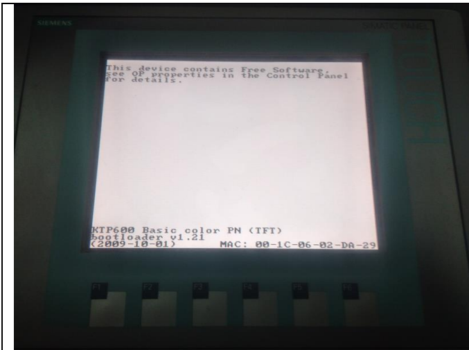
Fig.4 Turn the PLC trainer OFF by switching the power switch and turn it back on again. The shown screen shall greet you when it starts.
