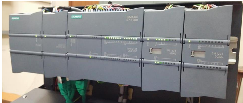
Fig.10: Our SIEMENS S7-1200 PLC rack. The central module is the processor along with IO and communication devices
