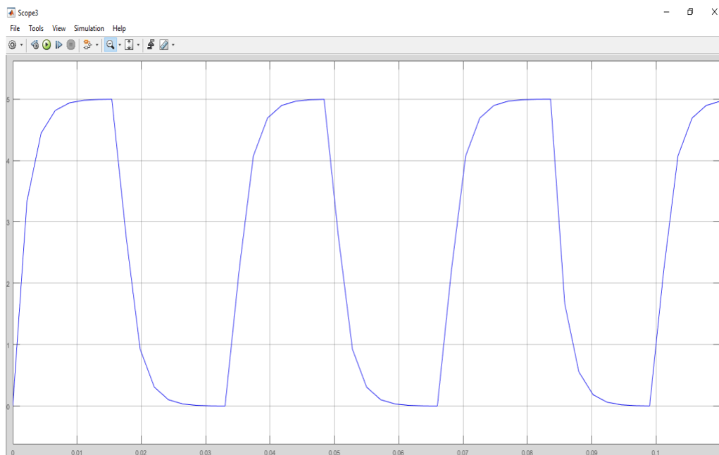
Series RC circuit response [v(t) \text{ vs } t]
